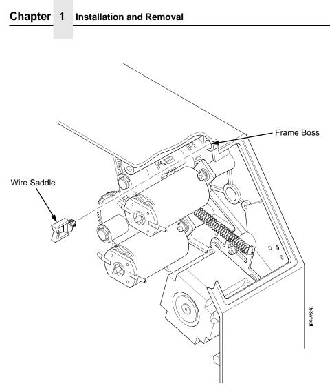
Figure 4. Inserting the Wire Saddle Into the Frame Boss
